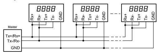
Control via RS485 4 wire bus (Optional Four-Wire Modbus Definition) as described as follows is optionally possible.
