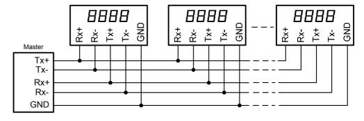
If the Modbus only consists of one master and one display as described as follows, in menu item 1 setting RS485 can also be selected.
