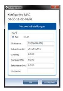
Enter the desired IP settings and click the 'OK' button. After successful configuration the following window opens:
